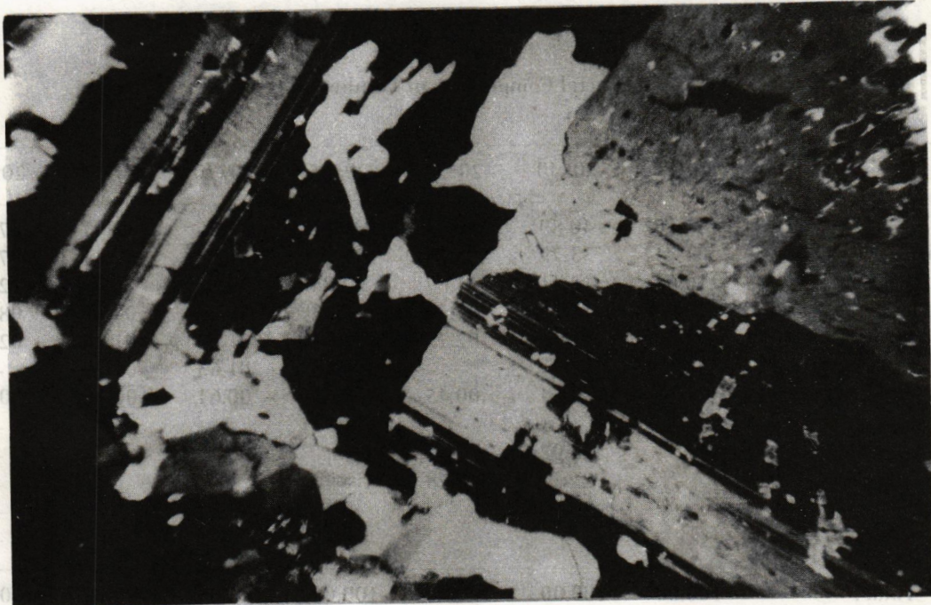
Fig 5: Photomicrograph of plagioclase showing albite - carlsbad twinning in porphyritic granite.
