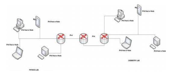
Figure 1 IPv6 to IPv4 Tunneling
